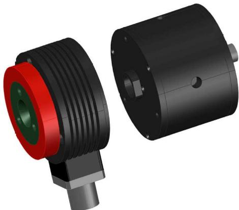
Fig. 1. General overview of the temperature-controlled filter holder with trap detector which in normal working conditions are mounted together.
